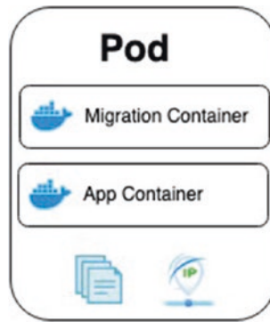
Figure 7-6. Diagram showing the pod architecture
