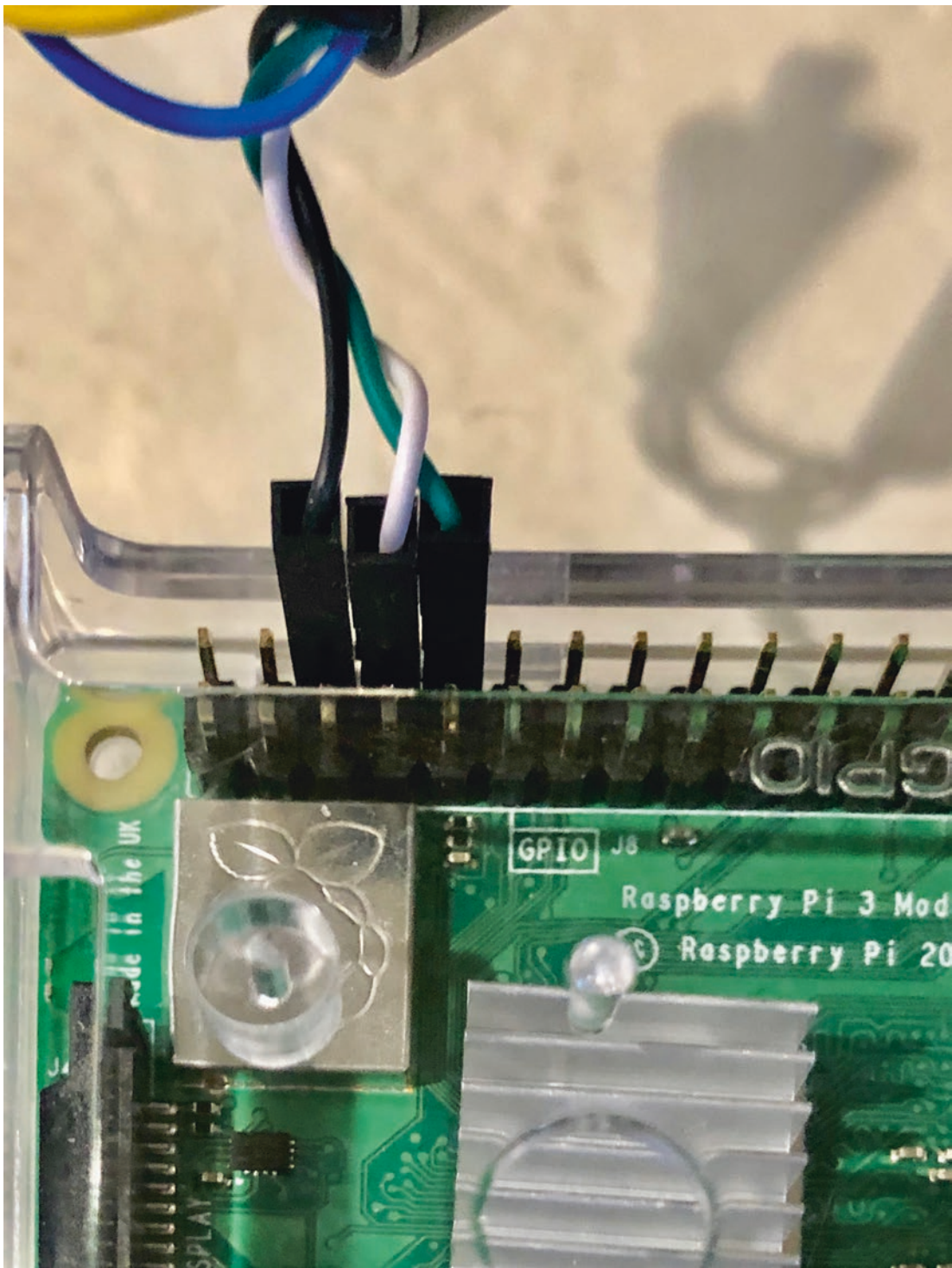
Figure 8-4. Our debug cable attached
