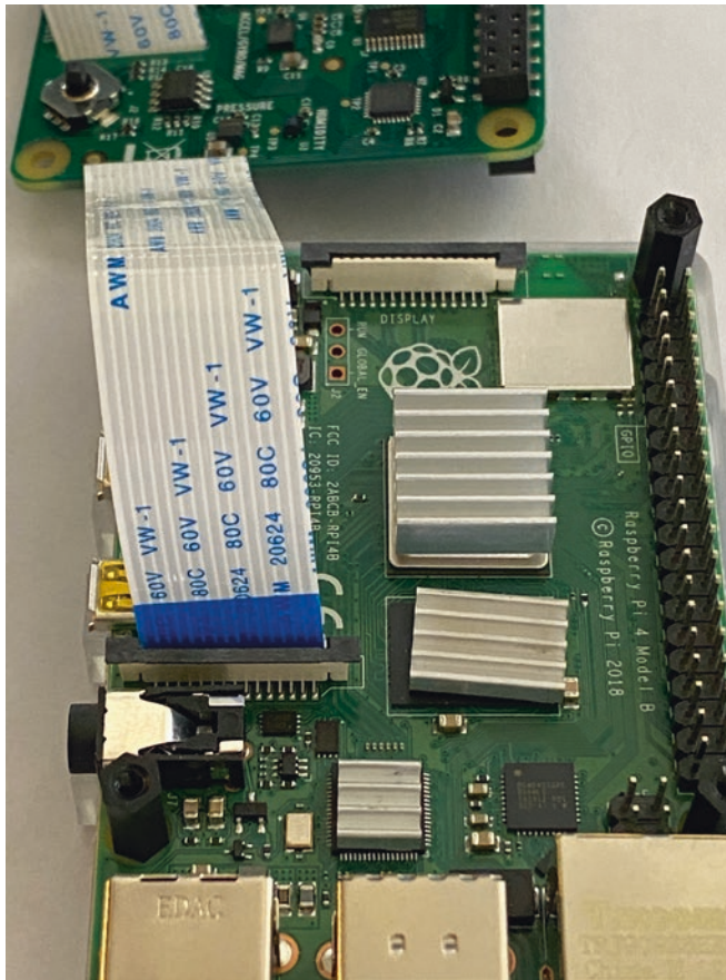
Figure 10-1. Showing the board where the connector is and connected all the way
