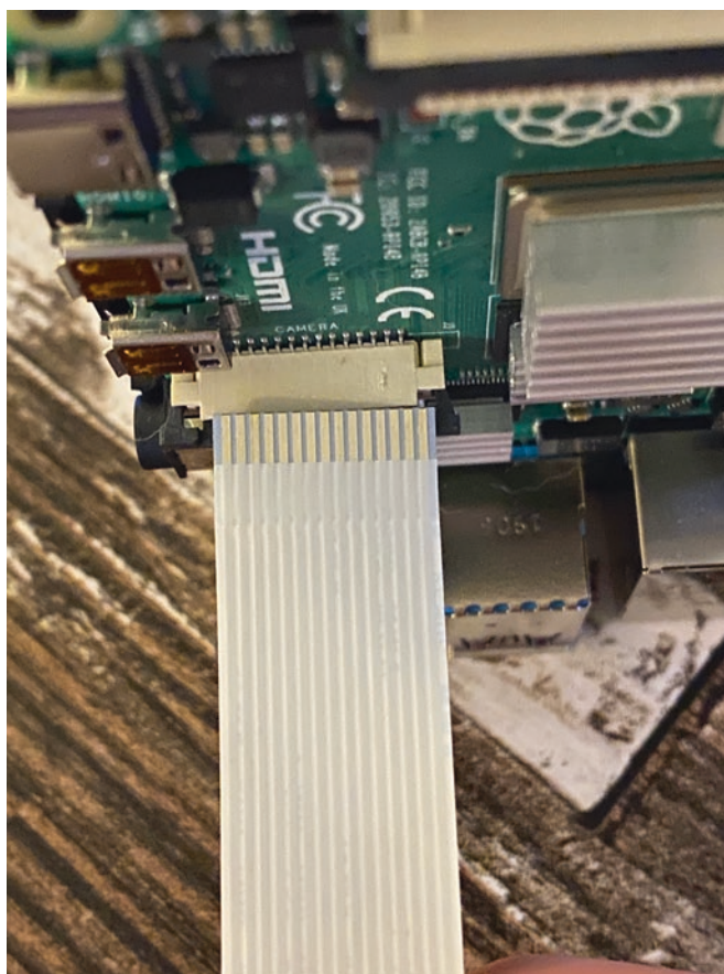
Figure 10-3. Camera connected to the board
