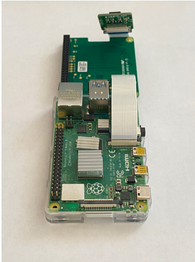
Figure 10-2. Camera connected to the board
