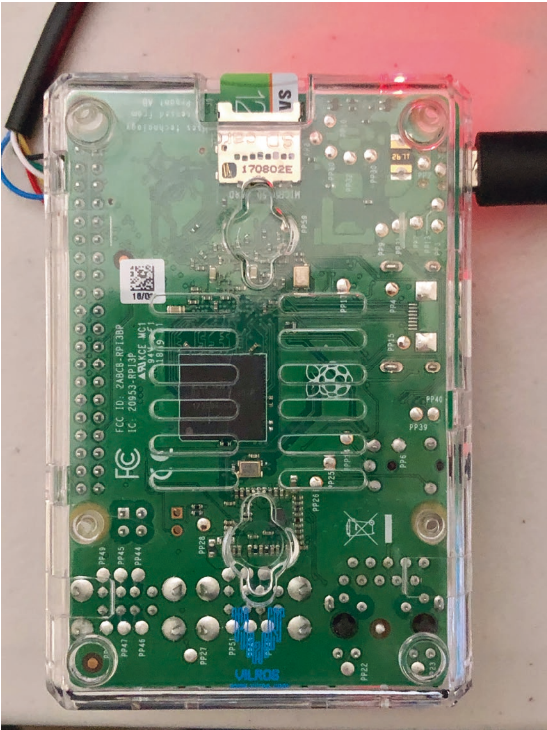
Figure 8-7. The microSD card installed into our Raspberry Pi
